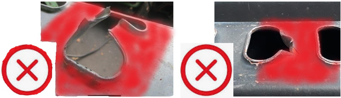
Fig 5. Cracked hook passage holes prohibited for lashing
